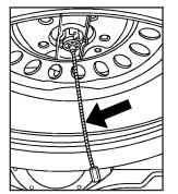
1. Check under the vehicle to see if the cable is visible. If it is not visible, see Secondary Latch System on page 436.
